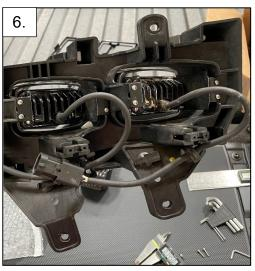
7. Using the supplied wire harness adapter, connect the adapter to the light and OEM wiring. The same functions will power the lights...
